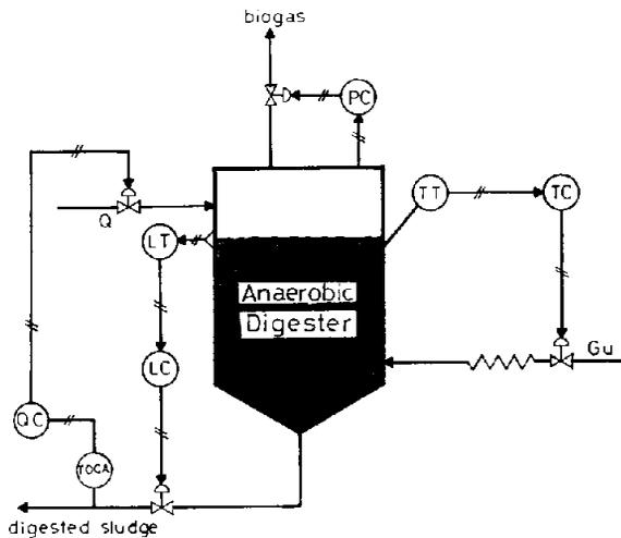
Fig. 11. Feedback control system for an anaerobic digester.
