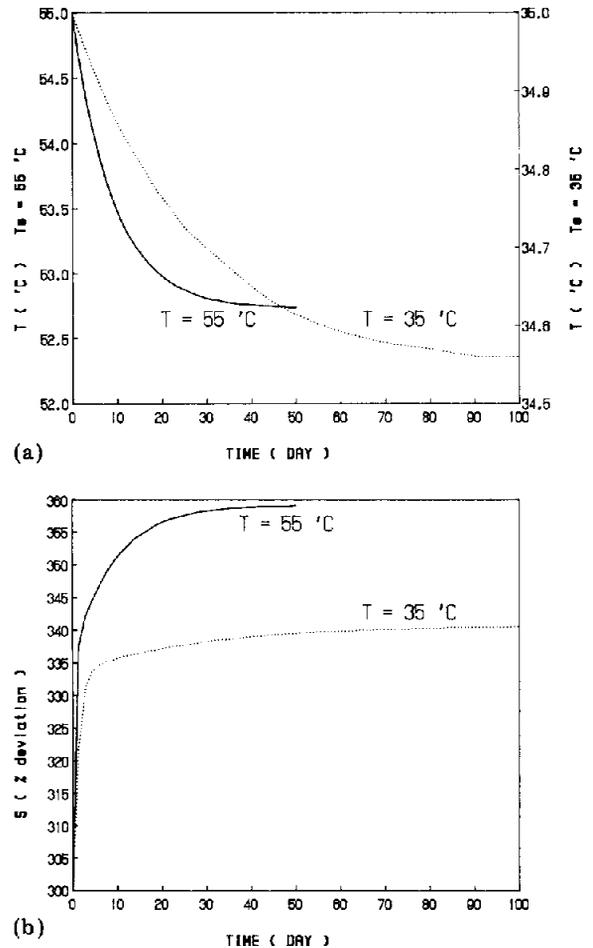
Fig. 3. (a) +10% step change in  $Q$  (inflow rate): effect on temperature; (b) +10% step change in  $Q$  (inflow rate): effect on bioconversion.
