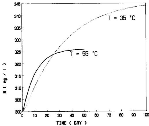
Fig. 5. -10% step change in  $T_0$  (inlet temperature): effect on bioconversion.
