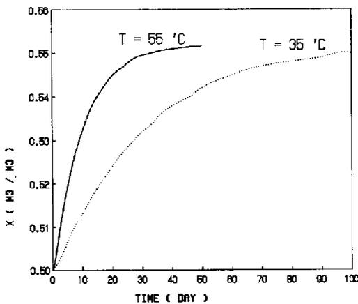
Fig. 6. +10% step change in  $S_0$  (inlet concentration): effect on biomass.
