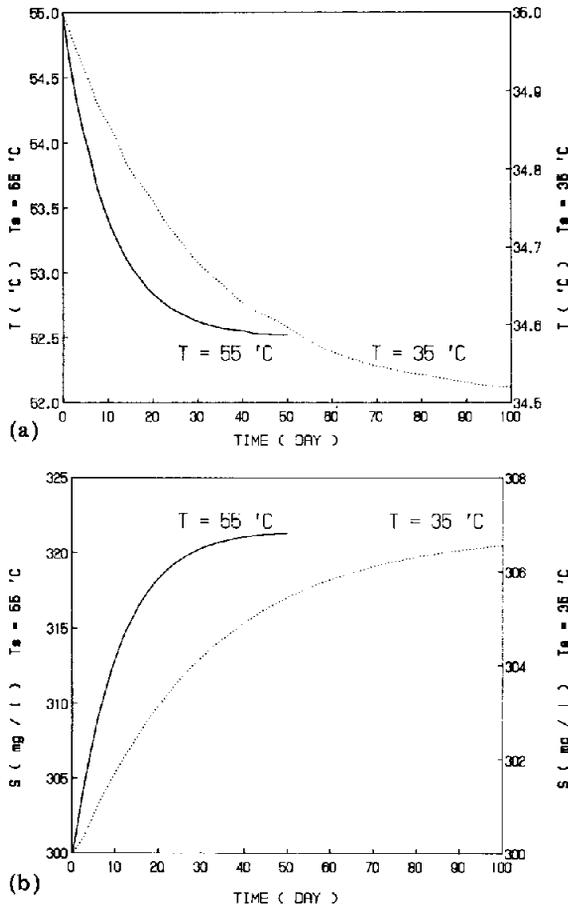
Fig. 2. (a) -10% step change in  $G_u$  (heat injection): effect on temperature; (b) -10% step change in  $G_u$  (heat injection): effect on bioconversion.
