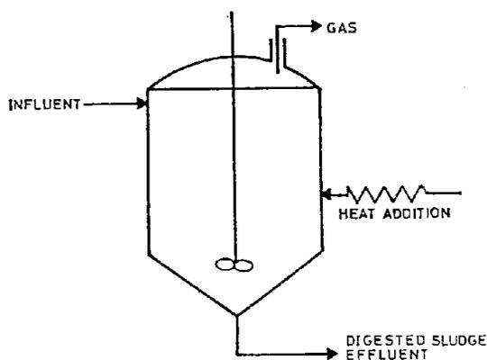
Fig. 1. The anaerobic digester.
