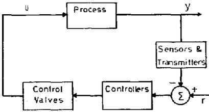
Fig. 9. Feedback control of a multivariable process.
