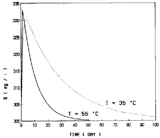
Fig. 7. +10% step change in  $S_0$  (inlet concentration): effect on bioconversion.
