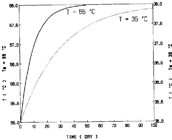
Fig. 4. +10% step change in  $T_0$  (inlet temperature): effect on temperature.
