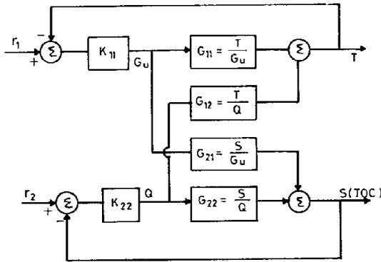
Fig. 10. Multivariable control of anaerobic digestion.
